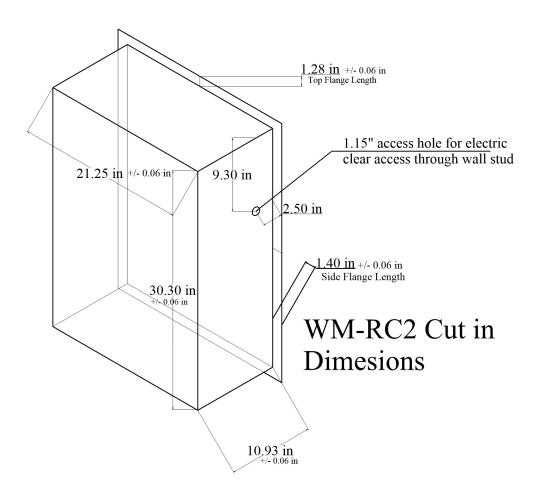
Wiring for your unit enters the unit through the side. When you purchased your unit you will have chose the left or right hand wiring option. The wire entrance is located 2.75 inches from the front and 21.25 inches from the bottom. The design intent is to have the power wire be fed through a piece of rigid conduit and then into a junction box.
