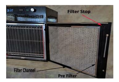
To remove or re-install lift the end of the prefilter over the filter stop and slide along filter channel
